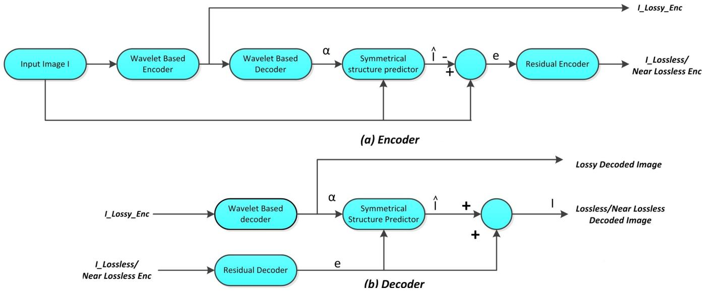
Fig. 1. Block diagram of proposed algorithm.
